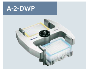
A-2-DWP 2-place deepwell plate rotor for plates up to 89 mm loading height. Max. speed 2,250 x g (3,750 rpm).
